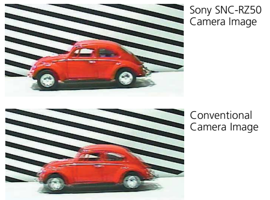
Fig. 3 Image Comparison Between the Sony SNC-RZ50 and a Conventional Camera
